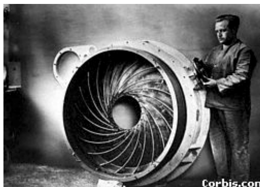
Figure 3. A very large iris diaphragm (from a telescope).
